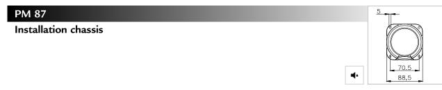
PM 87: Compact, highly-effective speaker for recessed installation. Especially suited for installation in sound columns.
